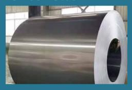
Silicon steel is undoubtedly the most important soft magnetic material in use today. Applications vary in quantities from the few ounces used in small relays or pulse transformers to tons used in generators, motors, and transformers. Continued growth in electrical power generation has required development of better steels to decrease wasteful dissipation of energy (as heat) in electrical apparatus and to minimize the physical dimensions of the increasingly powerful equipment now demanded.
