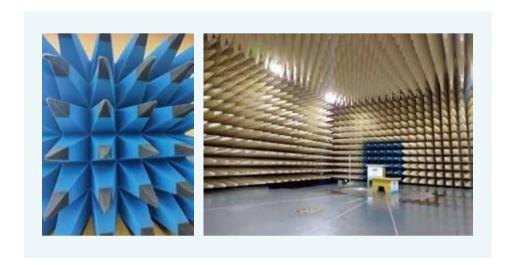
Polyhydrogen ester foam cone absorbing material
