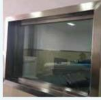
To provide viewing of the patient in the x-ray room while providing protection to the operator, lead glass viewing windows can be furnished in the barrier. Lead glass can be installed in multiple layers so as to provide a lead equivalency to the lead in the wall in which it is installed.
